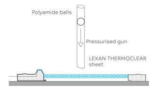
A test sample is clamped into a metal frame and polyamide balls of varying diameters are fired at the surface of the sample using a pressurized airgun.
