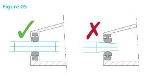
In general the total rebate depth for each profile should include a minimum of 20 mm sheet edge engagement and an allowance for thermal expansion.
