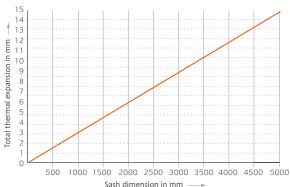
Sash dimension in mm — Allowance for thermal expansion must be made for both the length and the width of the LEXAN THER-MOCLEAR sheet. The recommended allowances for various sheet dimensions are outlined in the graph. The sheet must be trimmed to allow for at least as much as the indicated thermal expansion.
